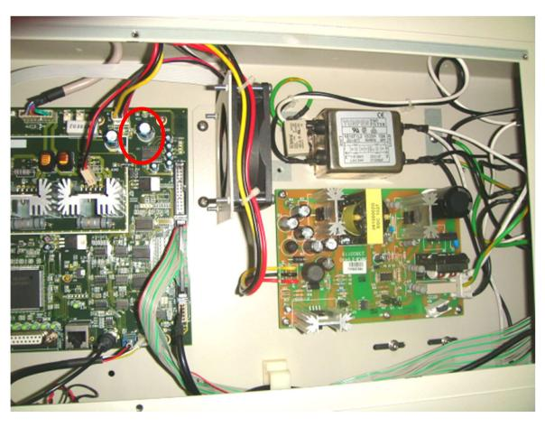
4. Loosen five screws to remove the power board (see picture below)
