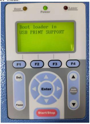
Step .2 Connect the USB cable between PC and Laser machine then run firmware uploader
