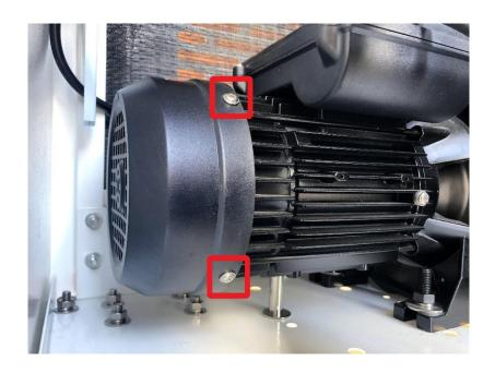
2) Use a screwdriver to turn the cooling fan at the back of the motor several turns to the arrow as picture. This may help dislodge any shaft blocks.
