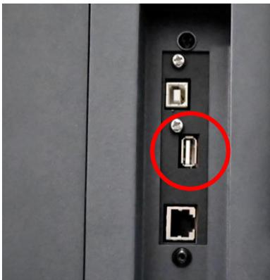
The USB storage port allows you to transmit data from a USB flash drive. Please refer to Chapter 4.1.3 for more details on operations.
