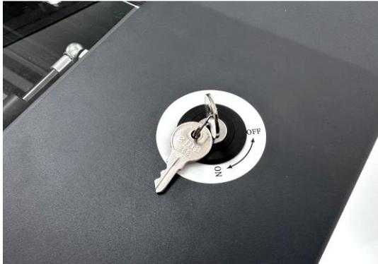
Turn the key-switch to the “ON” position BEFORE powering on the machine. If the key-switch is turned to the “OFF” position, the laser will be disabled meaning that the laser will not fire although the XY motion system will still move. The laser firing will need 8-10 seconds to warm up if turning to off, and turn on later, therefore, please wait 10 seconds before pressing STRART button for laser work.
