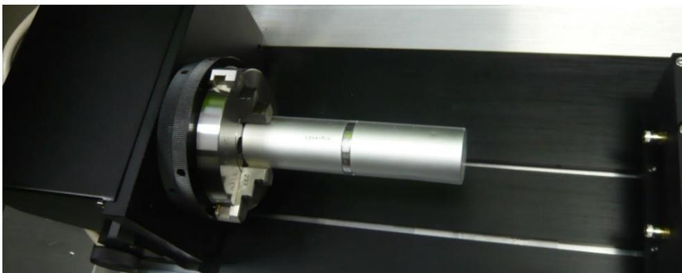
The clamps on the rotary attachment can be detached and reverted for better fitting of objects of different sizes. Note that the clamps should be assembled by lining up the correct numbers.
