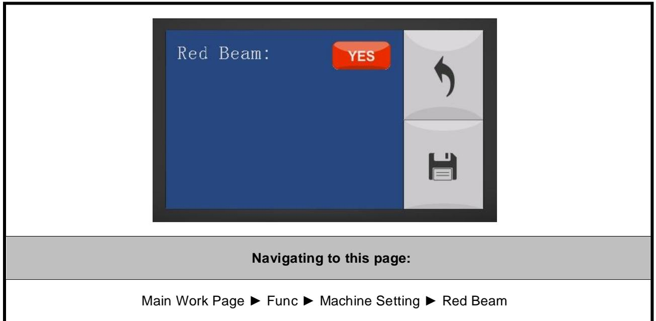
The Red Beam Page allows you to turn on or off the red dot laser pointer on the lens carriage. Enabling this function will indicate the exact area the engraving laser will fire upon.
