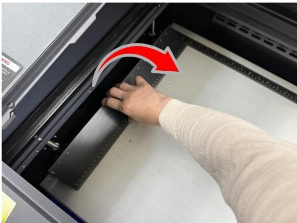
Step 2. Rotate the ruler 180 degrees to switch to the Imperial system.
