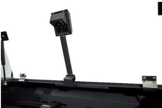
SmartEYES™ CCD on the top lid enables capturing the entire working area of the machine, making positioning easy. Please refer to the following instructions for operation.
