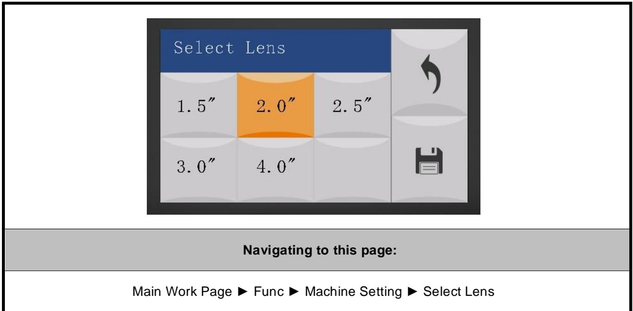
The Select Lens Page allows you to modify the lens settings after you have changed to a different focal lens. Remember to save your settings after you have made the proper changes. After that, pressing the Auto Focus button on control panel, the laser machine will conduct auto focus accordingly using the new lens setting.
