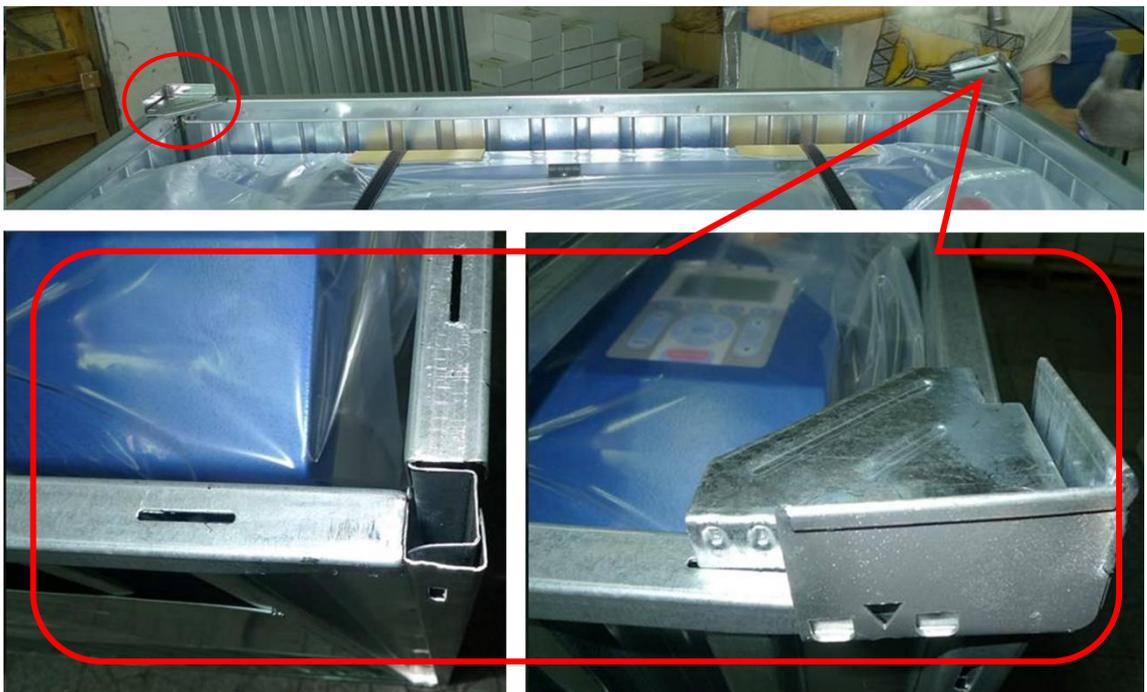
Step 5. Place the top cover on the top of the machine and fix it with the fixers.
