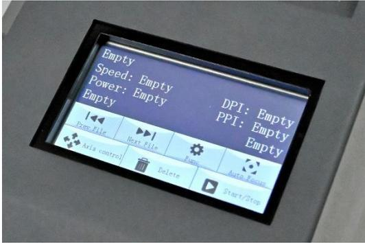
The 4" touch panel enables the user to manage files, adjust machine settings, and more.
