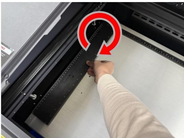
Step 3. Place the ruler back on the working table. The magnetic feature will ensure it is fixed in the correct position.
