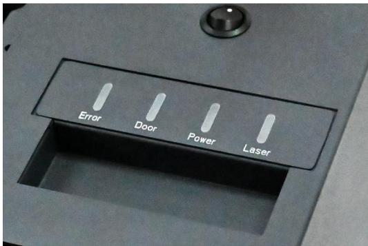
The four indicator lights on the LaserPro Spirit PRO Series Touch Screen are part of the system's safety interlock system.
