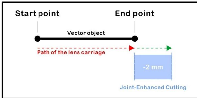
The lens carriage will move extend specific distance according to the object's shape when the lens carriage reaches the end point.
