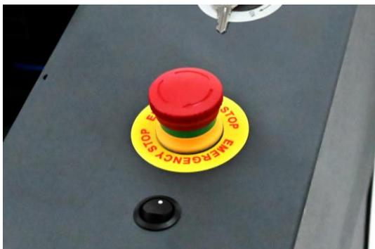
Press the button to stop the laser in an emergency. To reset this button, rotate it to the direction of an arrow.
