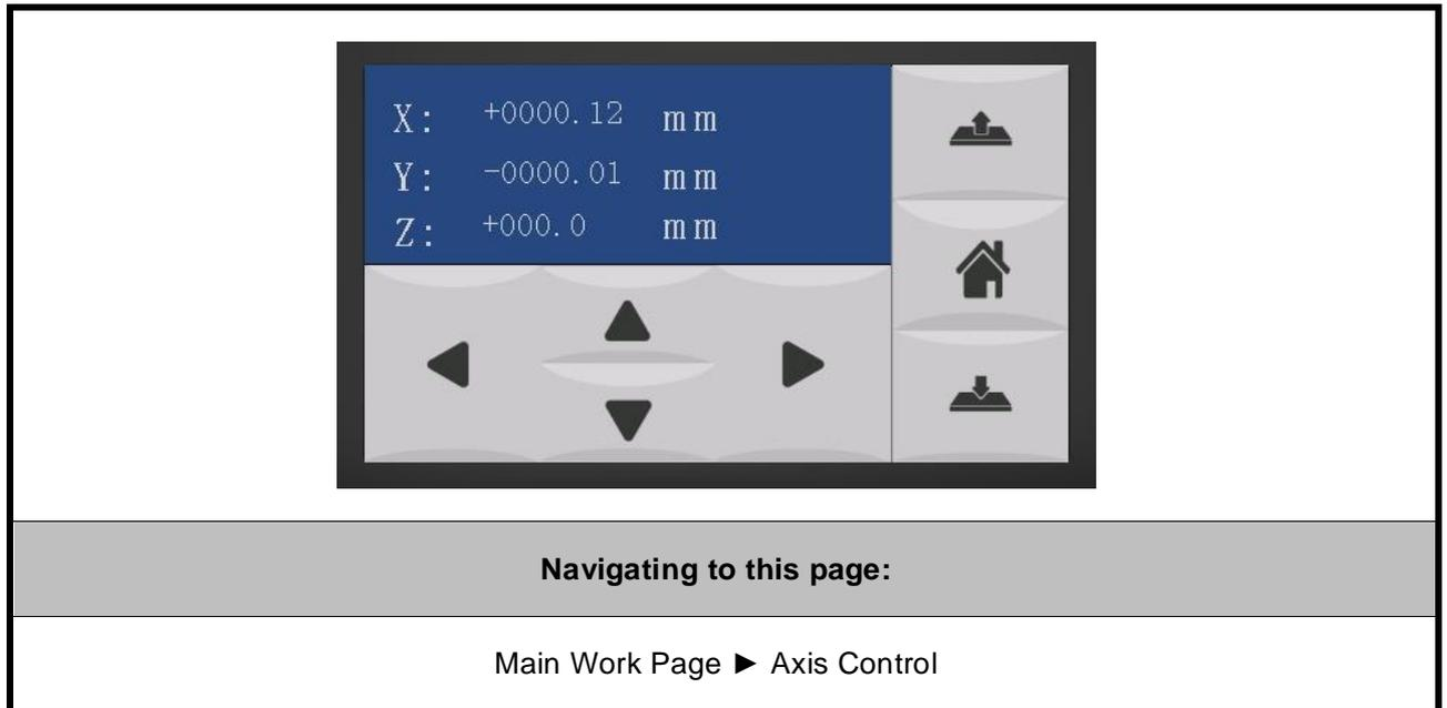
The Carriage / Work Table Adjustment Page allow you to manually increase and decrease the height of the work table (Z-axis). In addition, you can manually adjust the Y-axis and X-axis of the lens carriage.
