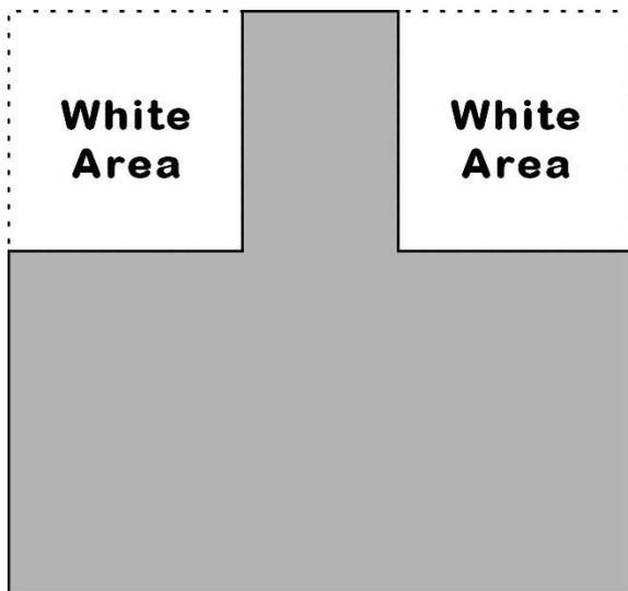
In the regular processing method, the lens carriage runs the job based on the maximum width of the entire shape. If the user enables the "Skip White" function in the print driver, the lens carriage will run the job based on the actual width of the shape, skipping the white areas.
