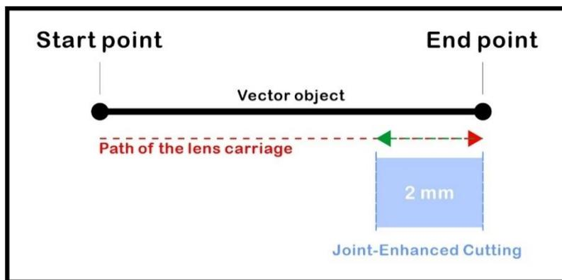
The lens carriage will move backward specific distance according to the object's shape when the lens carriage reaches the end point.
