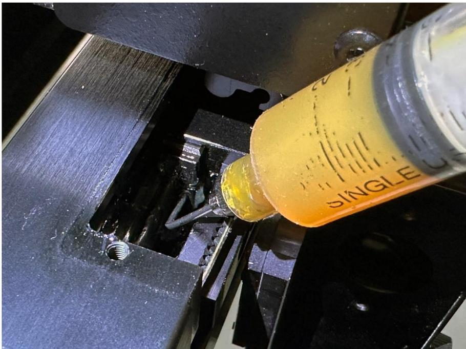
6. Repeat the step 5 till the grease is full out of the linear bearing
