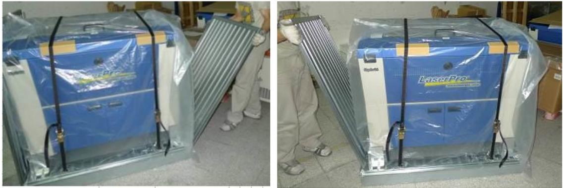
Step 4. Fix the four side boards by four corner brackets.
