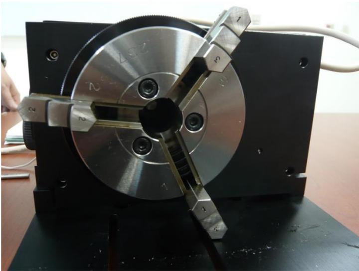
Please remember to lubricate the detachable clamps along the groove with machine oil regularly after each use.
