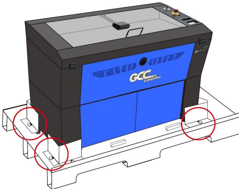
Step 10. Position the ramps as shown below and the machine can now be pushed off the base board via the ramps. (The ramps are found in a box within the crate)
