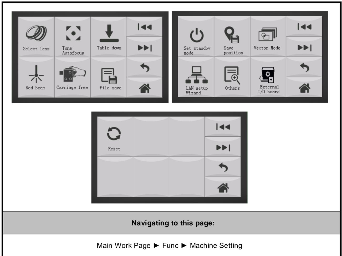
The Machine Setting Page allows you to access and modify various machine settings, including: Set Lens, Tune Auto Focus, Set Table Down, Red Beam on/ off, Carriage Free, select Command Mode, File Save, Set Stabby mode, Save position, Select Vector Mode, LAN setup Wizard, Scaling, Other, and Reset etc.
