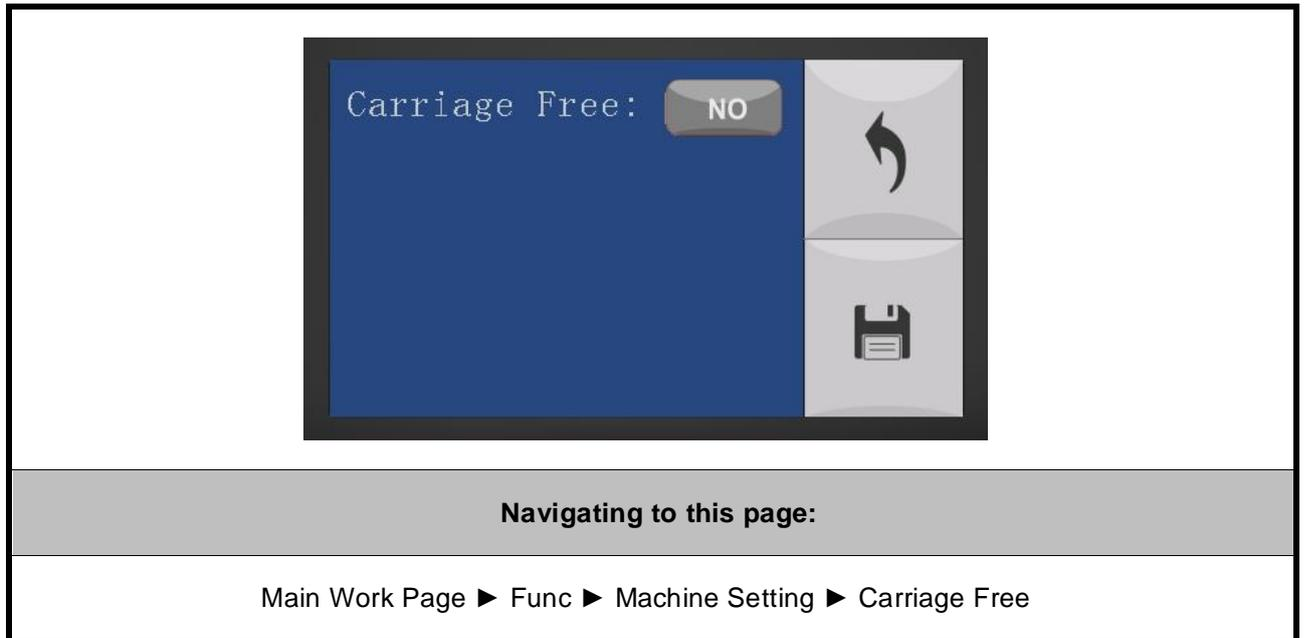
The Carriage Free Page allows you to decide whether the lens carriage to be locked or free for hand movement. If the Carriage Free setting is set to <YES>, then you will be able to manually move the lens carriage along the X and Y axis by hand with the top door open. Whereas setting the Carriage Free to <NO> will lock the lens carriage and movement or positioning can only be done by the Touch Screen arrow keys.
