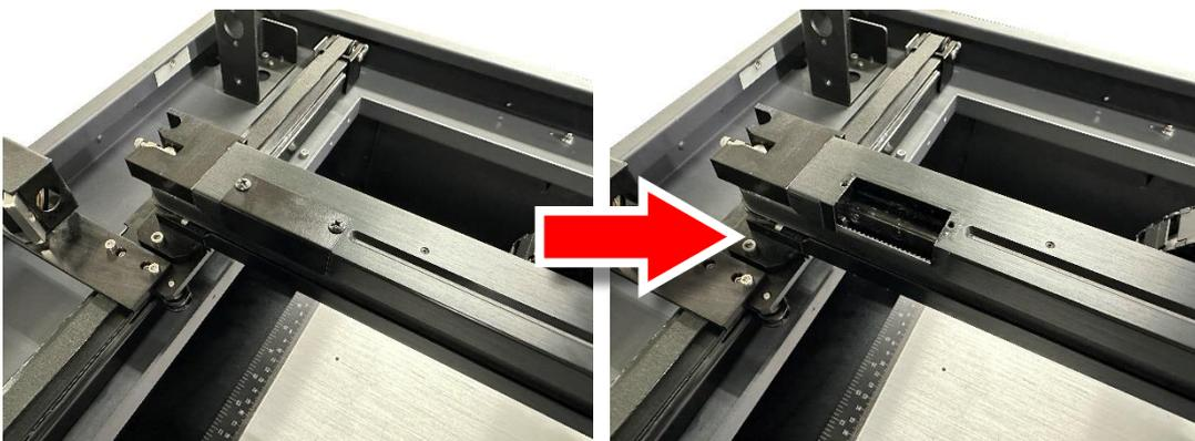
4. Move the lens carriage to the left side and make the injection opening can be shown from the lubrication slot
