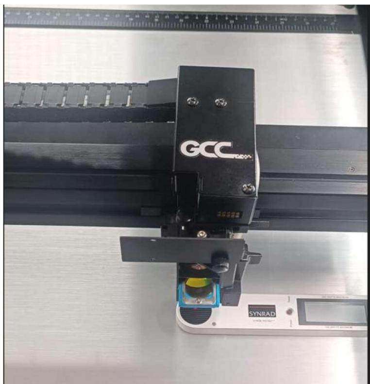
9. Fire laser (use default power level 90%, firing time 10s)
