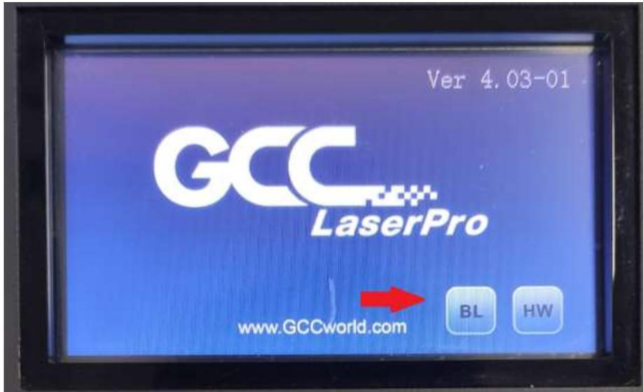
Click the “BL” icon to boot the machine into “USB PRINT SUPPORT” mode for firmware upgrades via USB cable.
