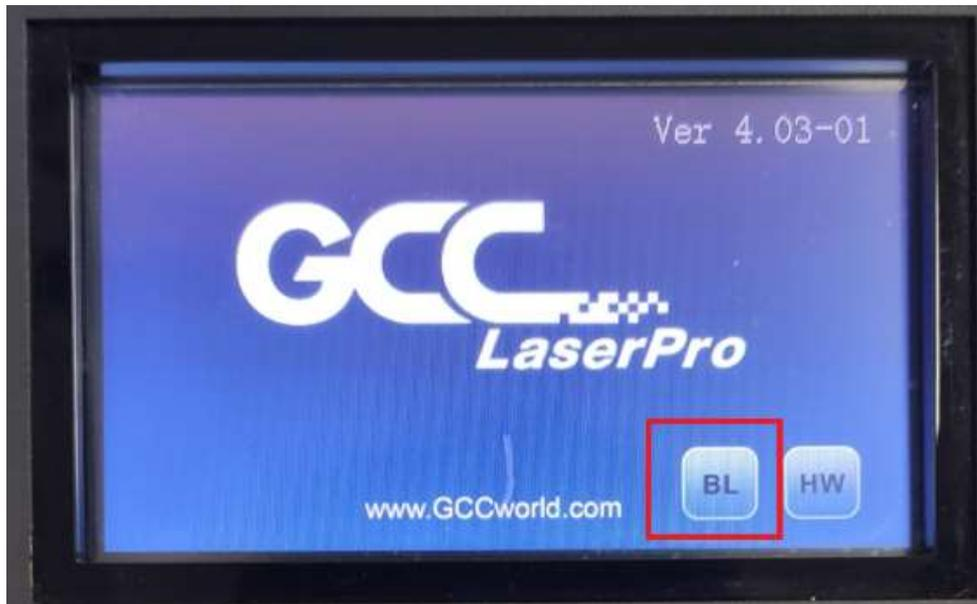
When the touch screen displays "Boot loader in USB PRINT SUPPORT," this indicates that you are ready to update the firmware.
