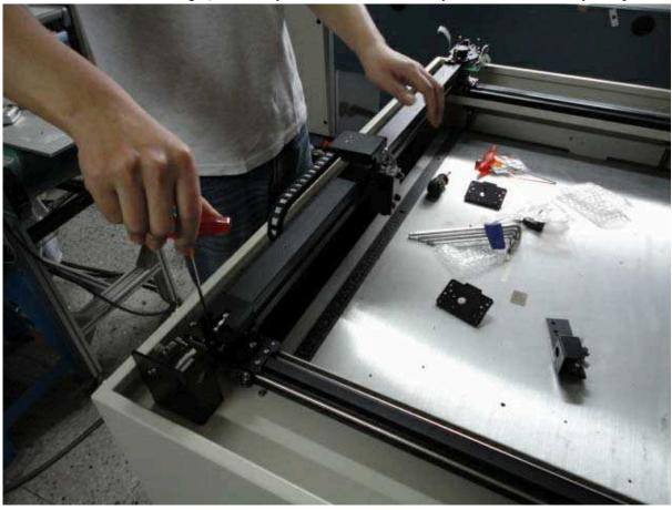
Connect the x motor flat cable to new x axis assembly and connect the air pipe (see red circle below) and tighten the three screws of x motor cover.
