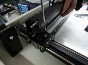
Move the whole x axis assembly to lower side (closer to your body) and then tighten all screws (two on the left and two on the right). This way can make sure the two y axis belts are evenly and parallel.
