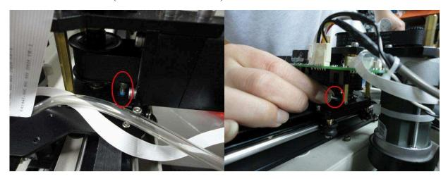
Then the alley key pass through the screw holes and reach the screw(see red arrows pointed below), but not tighten them yet.
