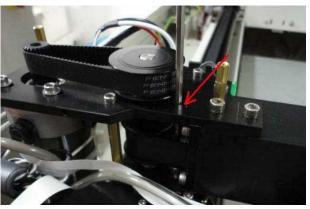
The right hand side of x axis assembly is easier to reach, but not tighten them yet.
