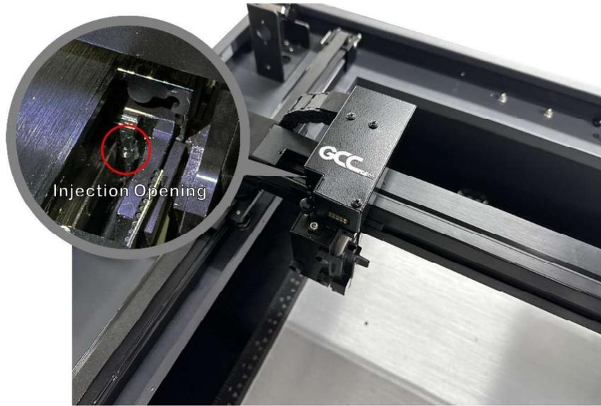
5. Insert the Grease Syringe into the injection opening, then Inject 0.1ml of grease to the injection opening inside the linear bearing, and move the lens carriage to smooth the grease and movement
