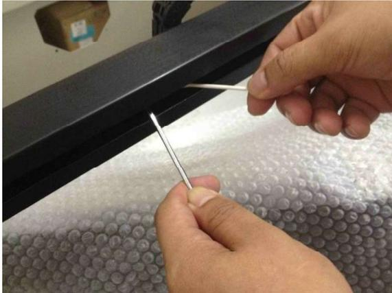
10. Use clean oil on cotton swab and then grease on linear guide (including top, bottom and surface of linear guide).
