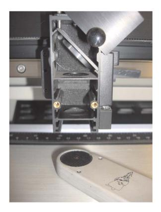
Place the **Black Target** of the power meter below the lens carriage so that the red dot is in the center. You do not have to be very accurate as far a center goes and focus does not mater as there is no lens.
