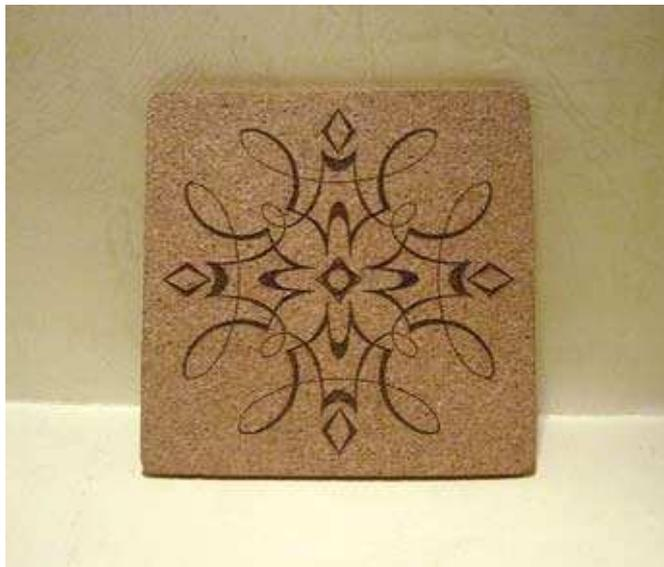
In these situations when there are raster engraving and vector cutting operations on a single project, the LaserPro C180II driver will interpret between raster sections and vector sections by the types of lines and line widths of your design. Areas of your design with line widths set between 0.001" (0.025 mm), 0.004" (0.1 mm) will be designate for vector cutting, and the other areas will be designated for raster engraving.
