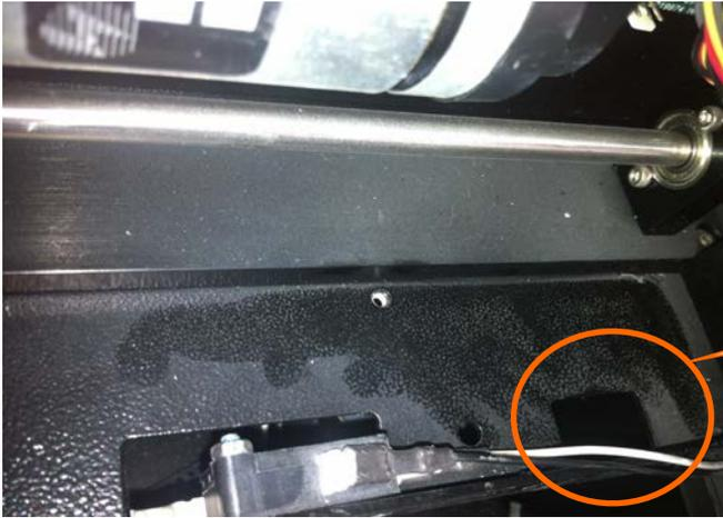
Insert the SmartGuard cable through the opening
