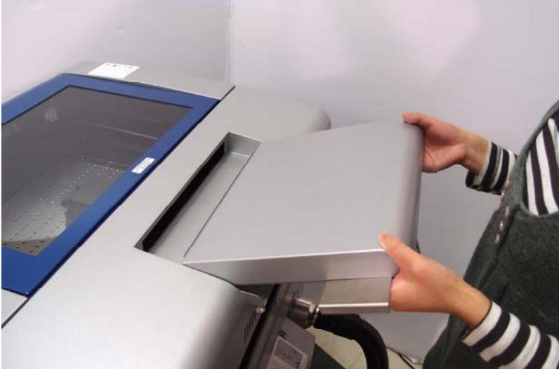
2) Tighten the 2 thumb screws by hand and the air exhaust connecting box installation is complete.
