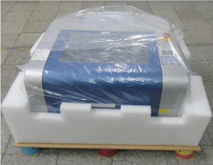
3) Place the top EPE on the machine and place the exhaust connecting box on to the EPE
