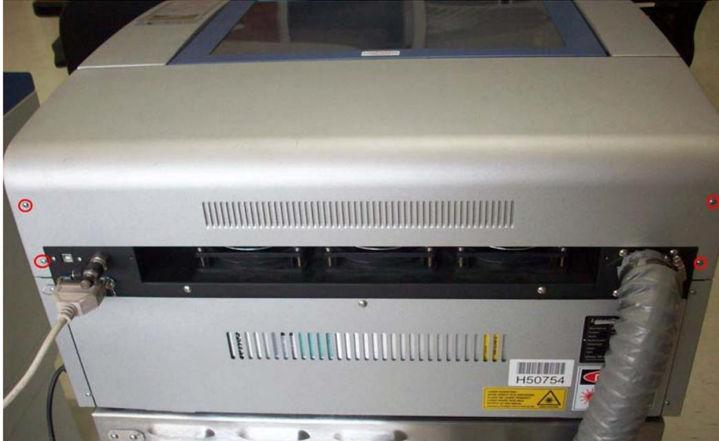
2. Remove shield cover by removing 6 screws. 3 screws on top and 3 screws inside (see below red circles).
