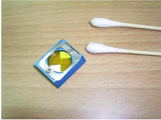
Make sure the lens is clean and dried before putting it back in the pen carriage unit.
