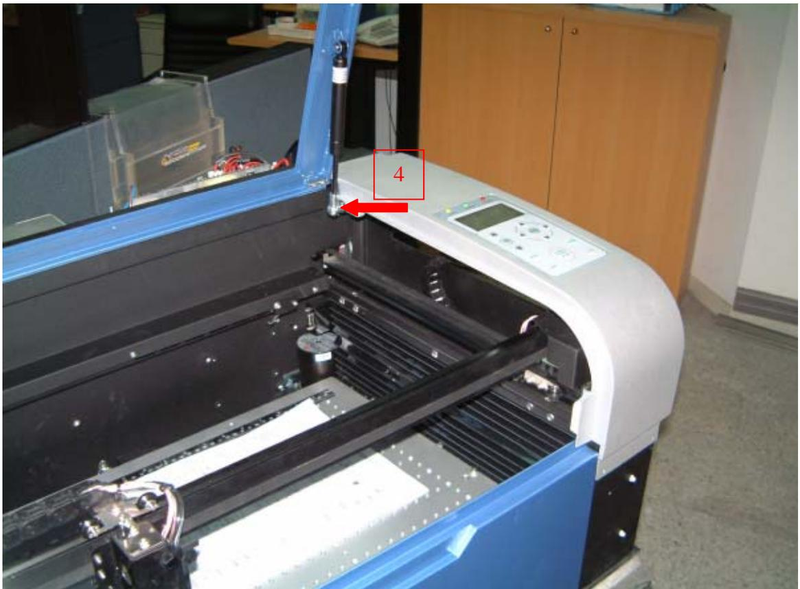
5. Dismount 4 screws of right top cover (where the control panel locates)
