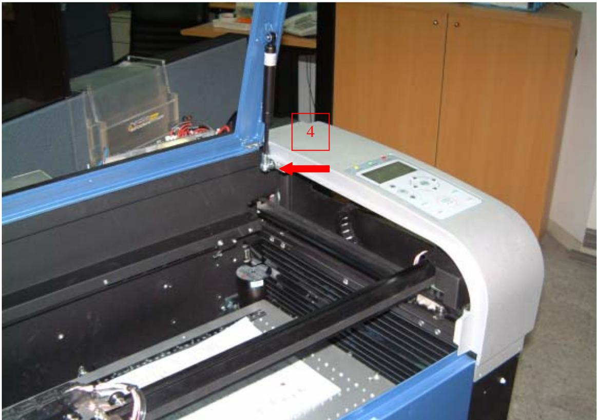
5. Dismount 4 screws of right top cover (where the control panel locates)
