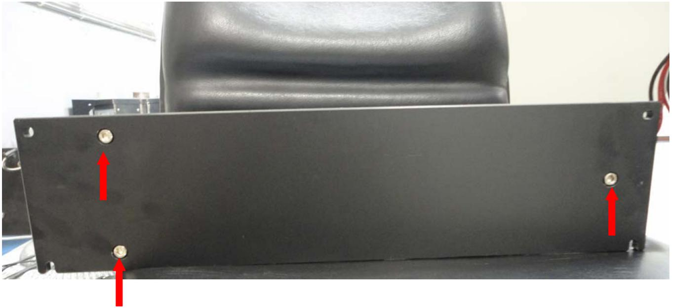
12. For changing bottom cooling fans, the laser tube need to be removed first and then the screws driver can reach the fan screws
