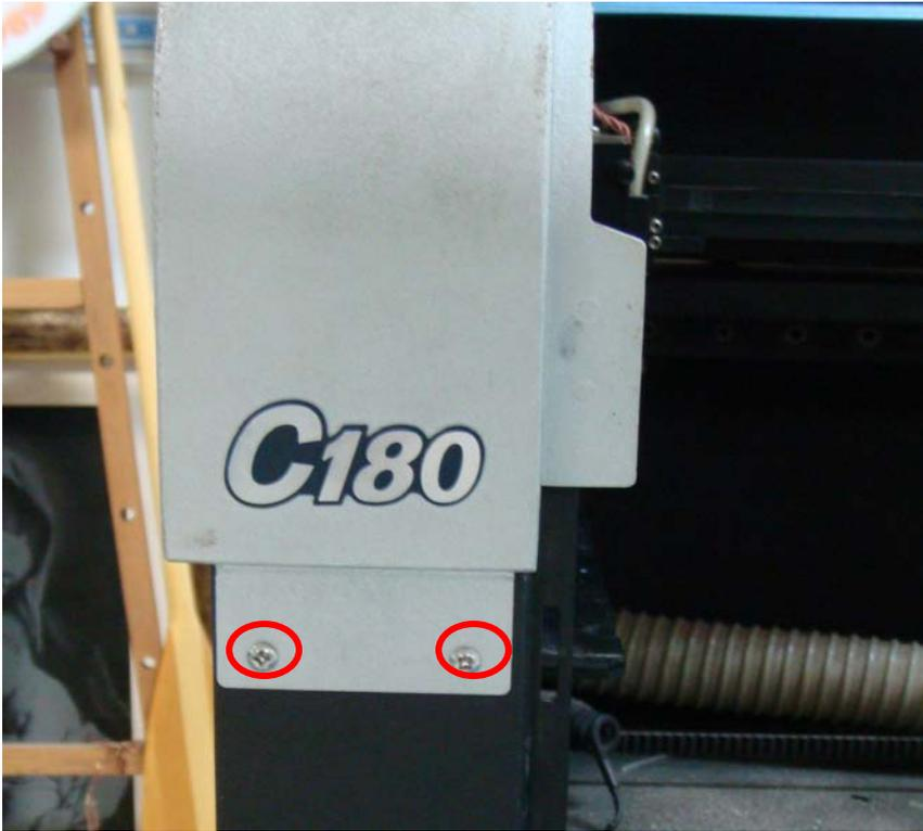
10. Then remove the back panel. There are three screws on front
