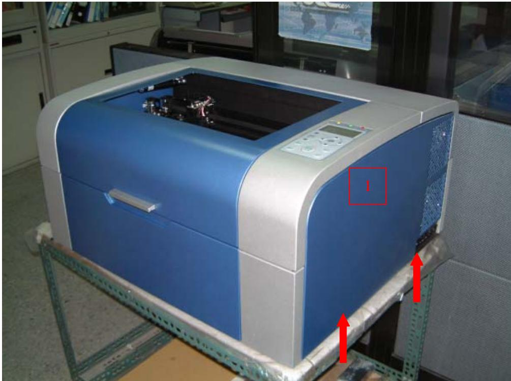
2. Dismount 7 screws (see red arrows below) and remove all cables connecting to main board and can change new main board.
