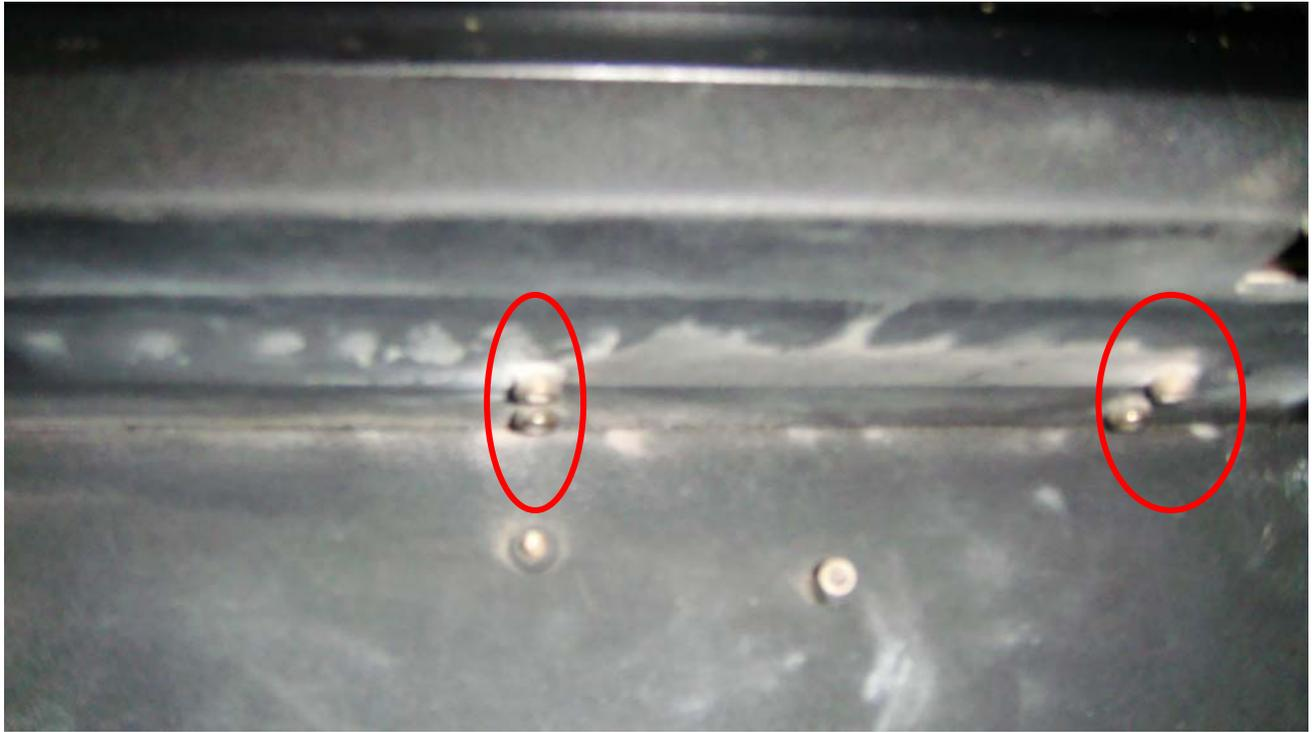
20, To move up the y axis synchronizer bar, the y axis belt need to be remove or loosen. To remove the left y axis belt will be easier by loosen the two screws of belt retainer (the red circle).
