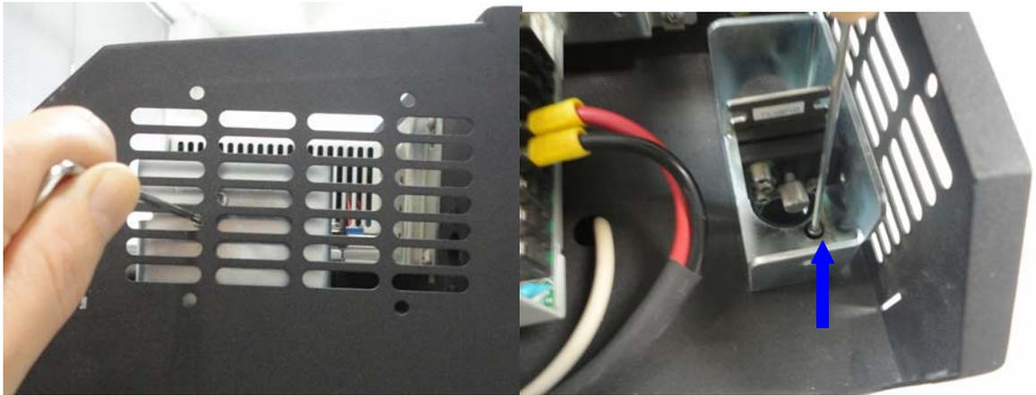
6. Remove the red beam mirror cable (see red circle) and remove the screw of mirror 1 dust cover (see red arrow). When laser tube is removed, the mirror 1 dust cover can still stay at same place.
