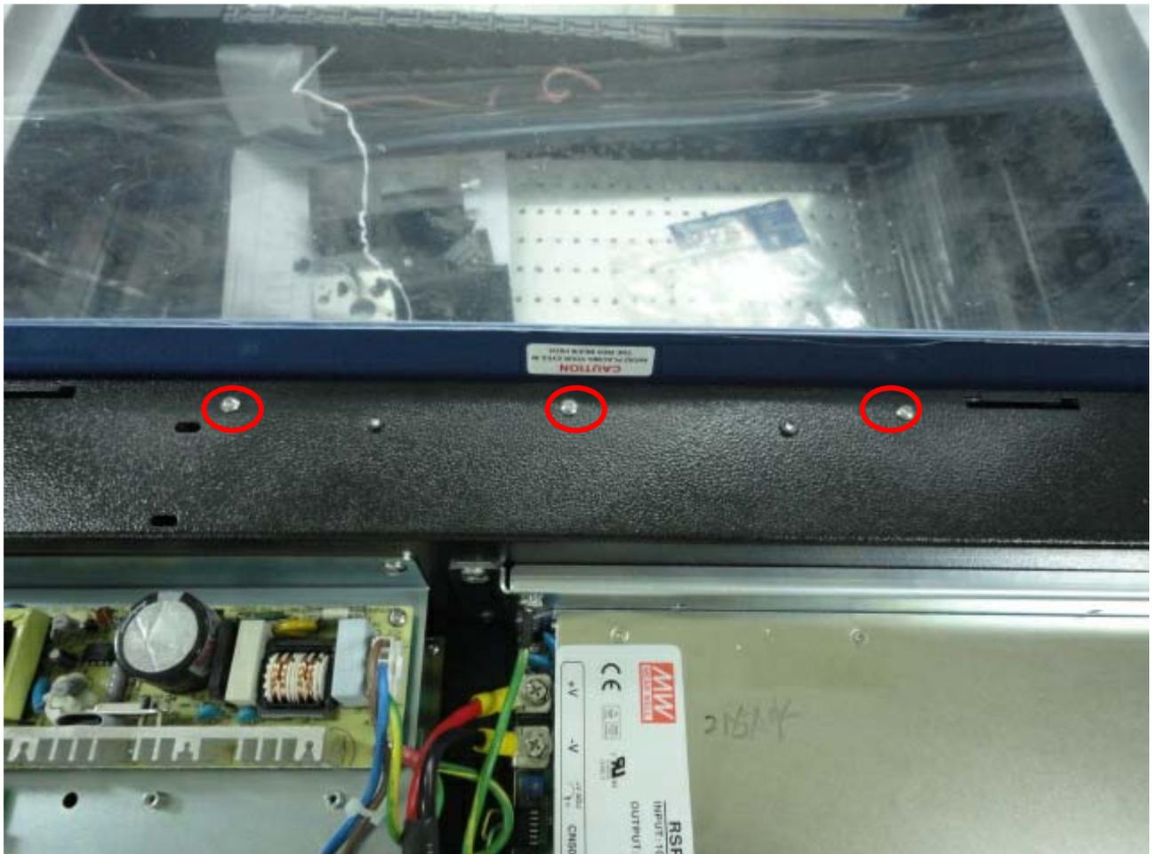
12. Then remove the working table. First remove two left screws
