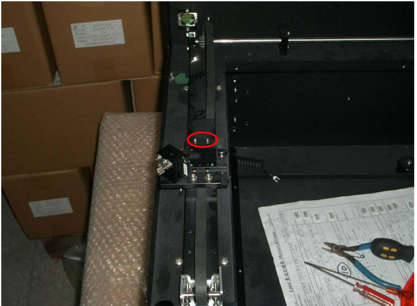
21. Now the whole y axis synchronizer bar can be move up a little. So the y motor belt is loosen also and can be removed.
