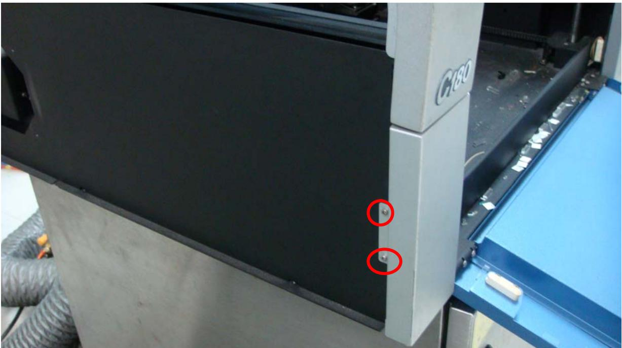
9. Remove left-front two screws
