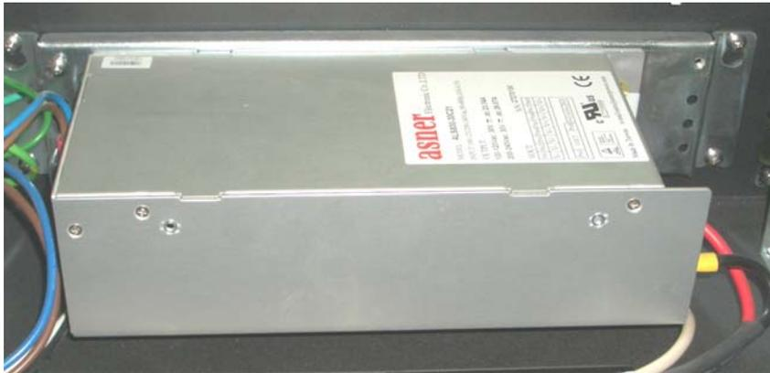
Power supply for 40w laser tube 24500064G, 1000W-48V (RSP-1000-48)
