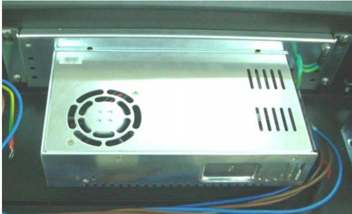
Power supply for 30w laser tube 24500032G, 800W-30V (ALS-800-30C21)
