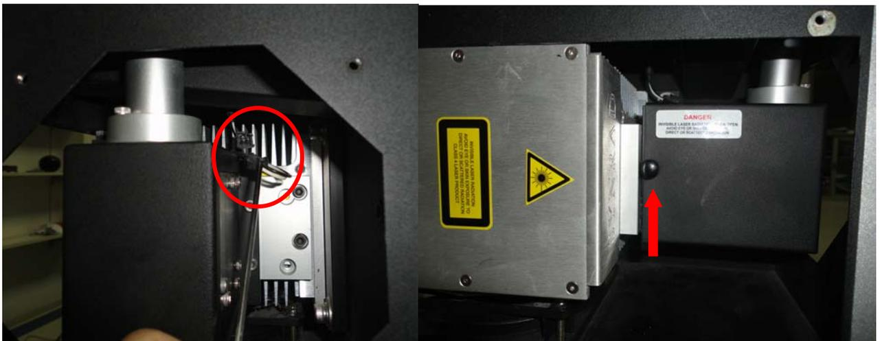
6. Remove the laser tube signal cable (red circle) and two screws of laser tube bracket (on left side).
