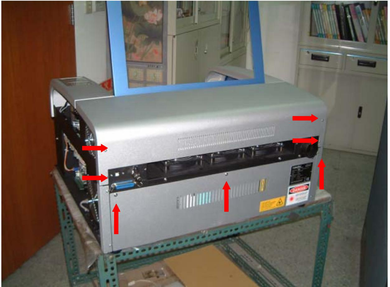
2. Remove left side cover: first remove the two screws on the bottom (red circles)
