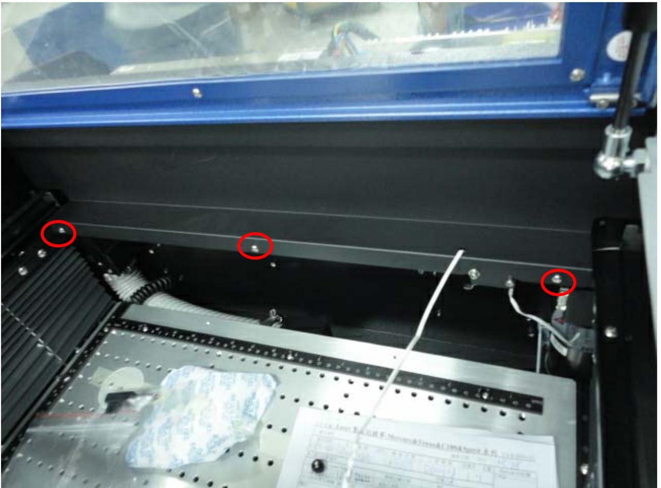
11. for back panel. There are three screws on top (from back side)
