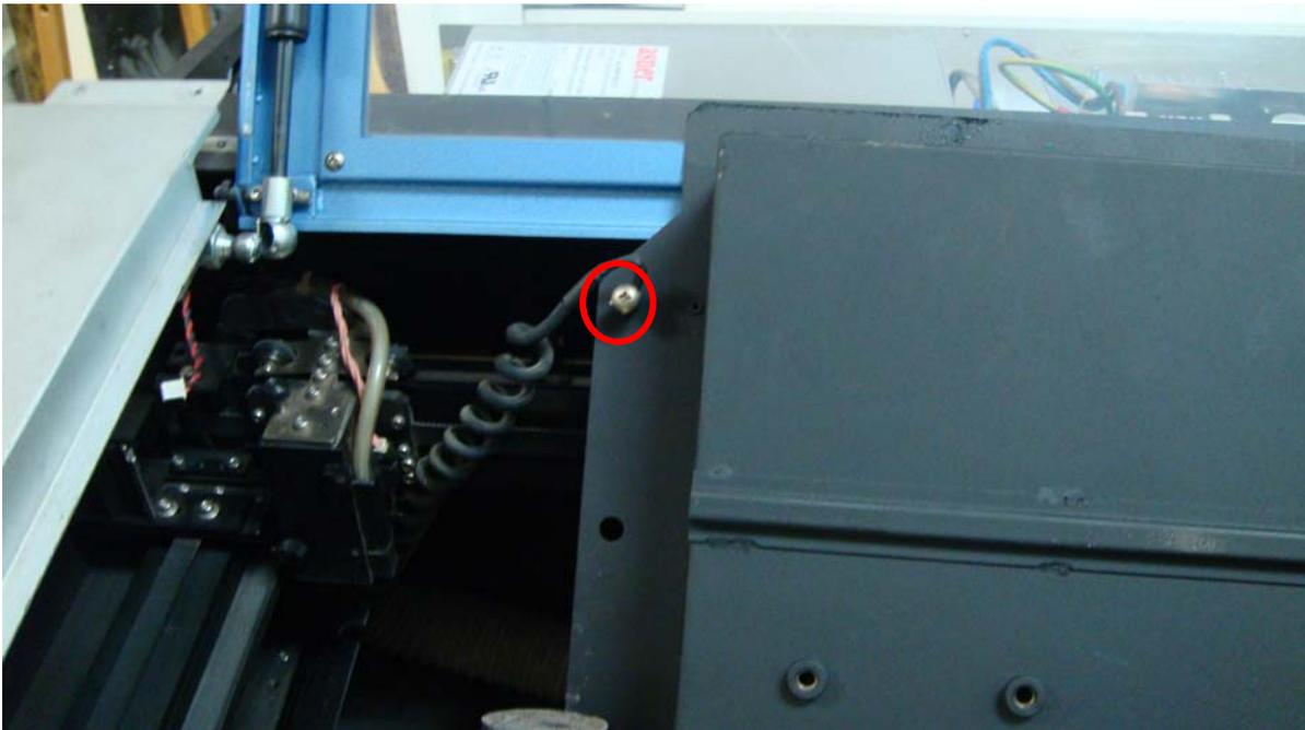
17. To remove the y axis synchronizer bar (the red arrows pointed) need to remove the screws of synchronizer bar holders and they are at the bottom (the yellow arrow pointed). The screws of synchronizer bar holders cannot be reached until the dust guide pipe is removed. The screws of dust guide pipe have 6 screws on top (the red circles)
