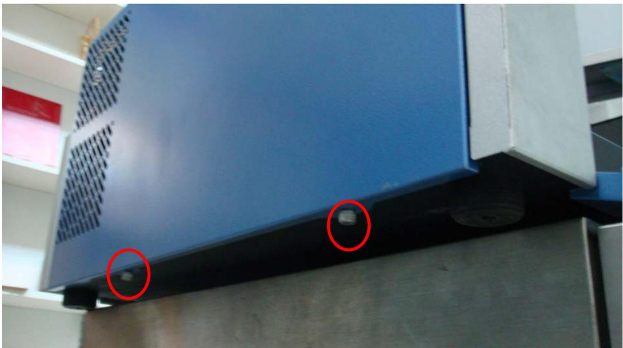
3. Then loosen screw and remove for the second mirror dust cover
