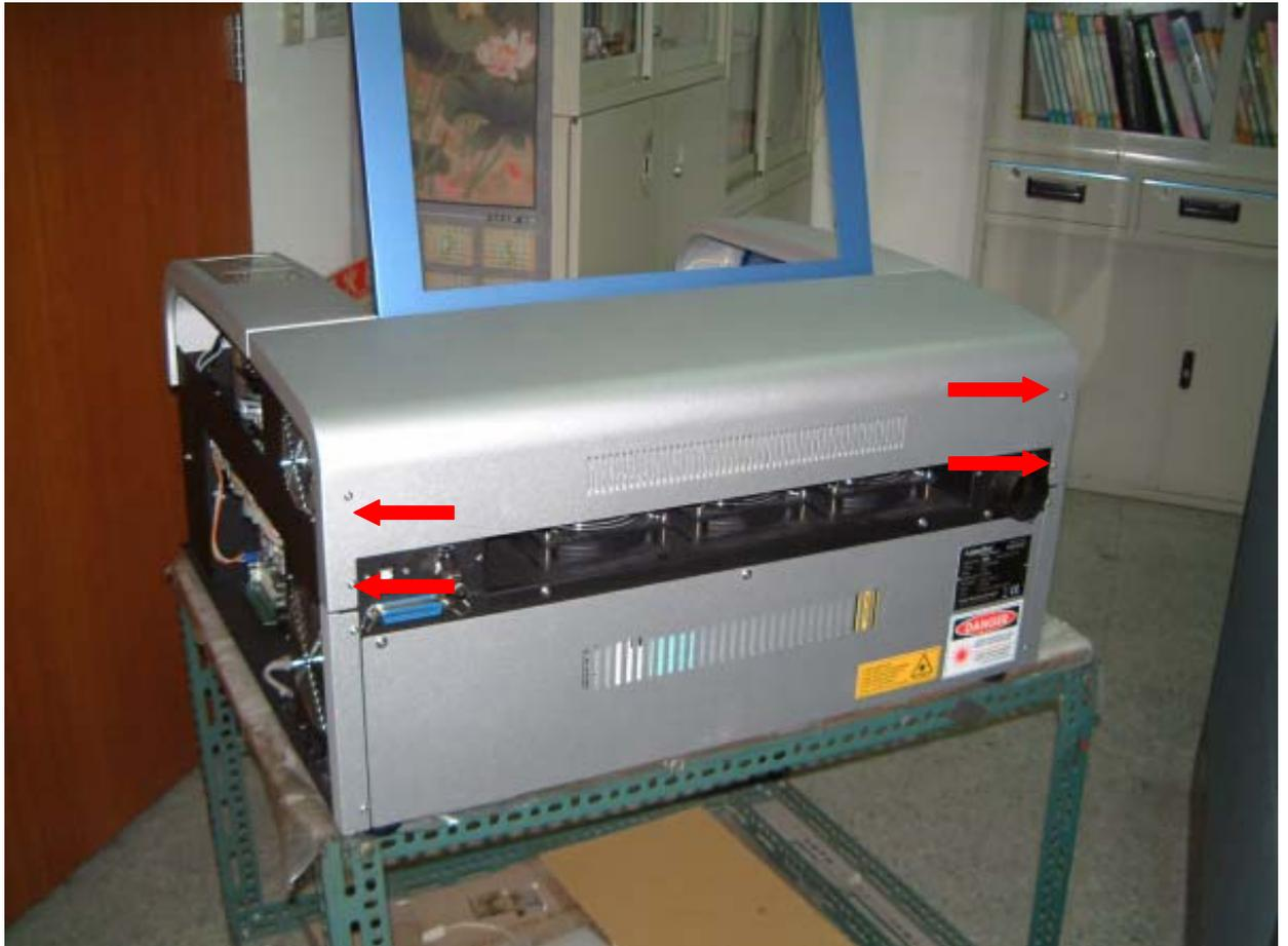
2. Loosen the screws and remove the two power supply AC side cable (red arrow)
