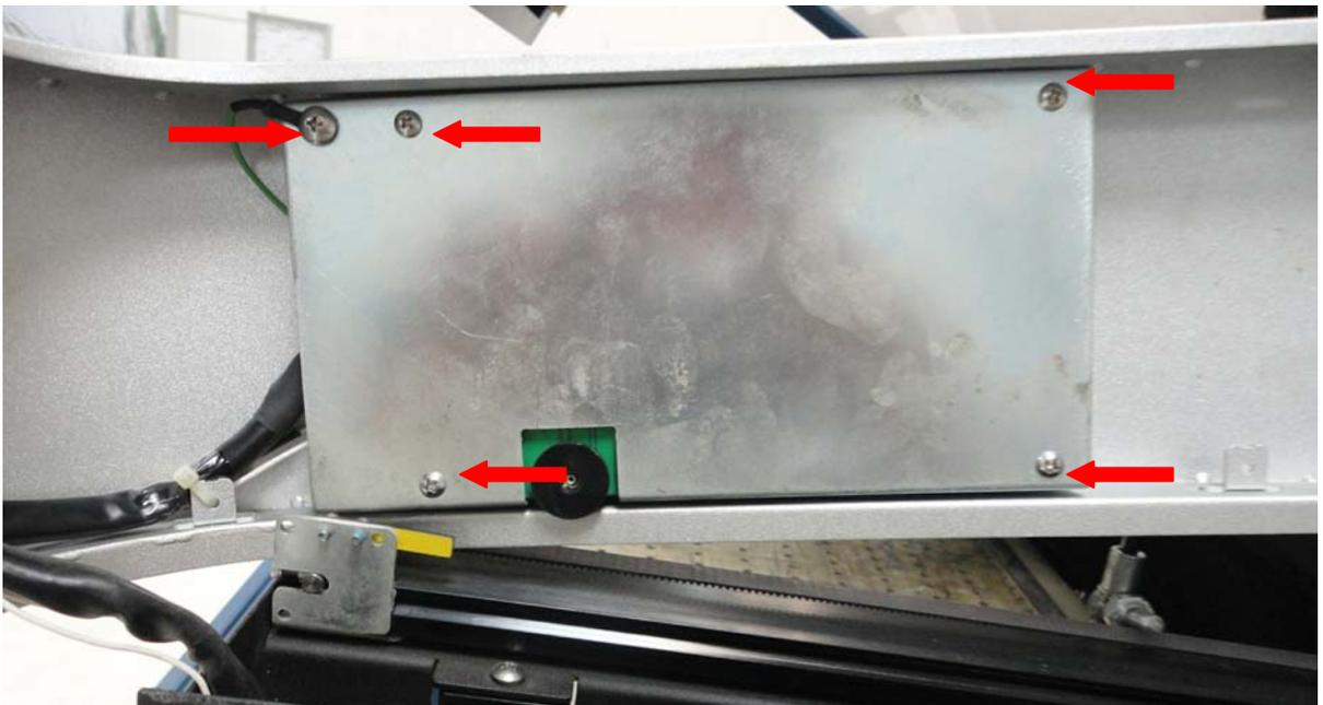
8. After control panel cover is removed, there are 4 screws needs to be removed and the four cables (in the red circle). Then the control panel can be removed and changed new one.
