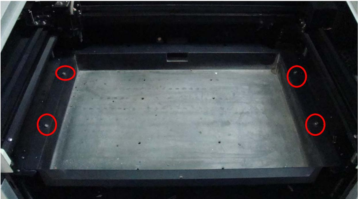
15. Then remove the dust pipe by removing screw
