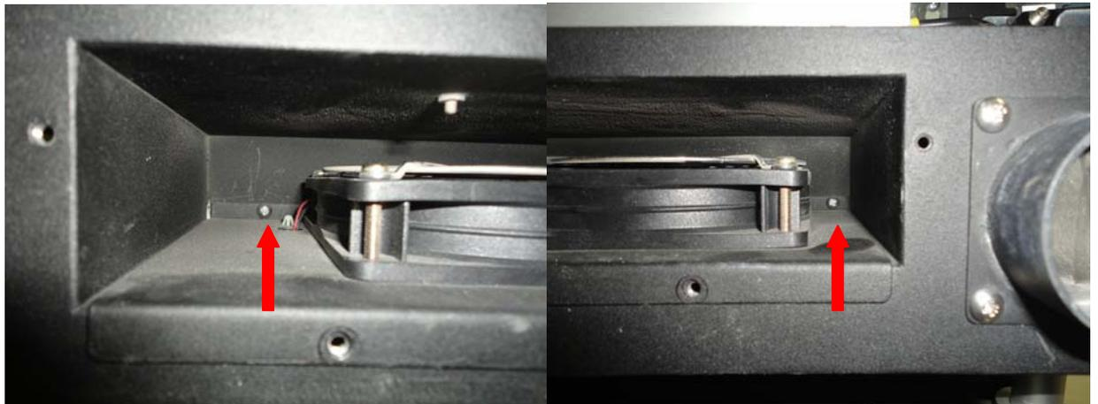
15. Then remove the 4 screws of that defective fan and then also remove the cable of those defective fans.
