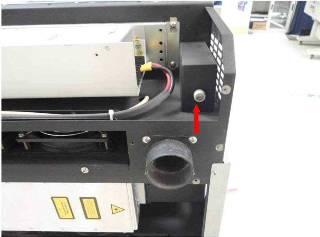
4. There are two screws for dust prevention pipe. The top screw (red arrow) can be reached easily, but the bottom screw (blue arrow) will be blocked by mirror 2 bracket
