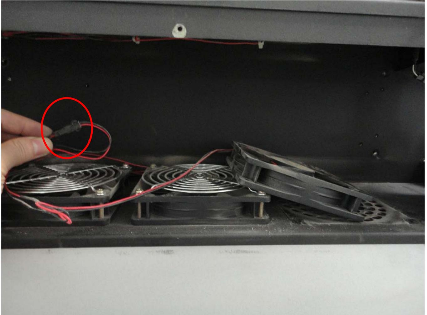
14. For changing top cooling fans, there are 6 screws need to be removed. See red arrows on below two pictures.
