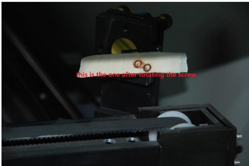
The new burnt spot is at top left of the first one, we should adjust a little back on both directions.
