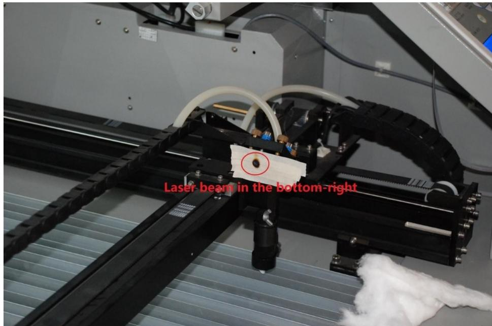
4. Move laser head to bottom left corner of working area, press Pulse button to shoot on the tape, shown as below.
