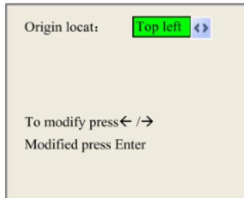
Press **Left** or **Right** key to switch option. We suggest setting same screen origin with the software, otherwise, graphics shown on screen will be mirror in X or Y direction with it shown in software, bring some confusion to operator.
