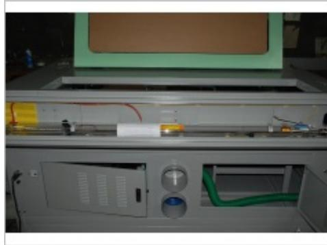
The laser output window should be about ½” (10-15mm) from the round porthole in the metal bracket on the mirror mount.
