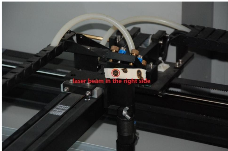
Check if two burnt spots are at same position and at center of circle of aligning plate at the same time, If not, repeat steps above until it's calibrated.
