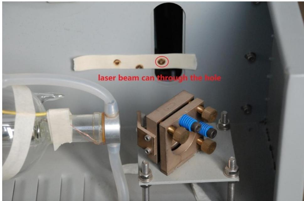
Burnt spot should be in range of the hole. If not, you should adjust base fixing screws to move mirror left or right, then check again, and do more adjustment if needed, until it's calibrated.
