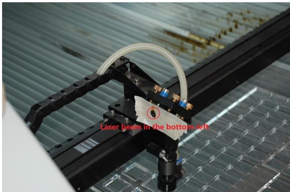
Check if four burnt spots are at same position and at center of circle of aligning plate at the same time. If not, check and calibrate laser route to all 3 mirrors again.
