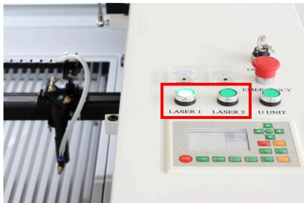
This button only enables laser operation. It does not actually switch on the laser until the rest of the control system is calling for laser power.
