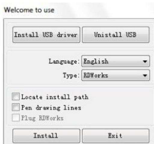
1. Click **Install USB driver** button to install communication driver for control system.
