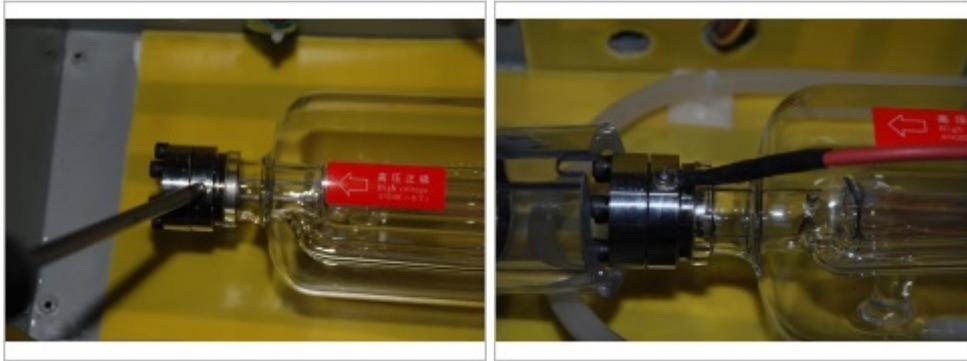
Connect the negative (yellow) wire to the cathode (-) side of the laser (the side facing the angled mirror). This side does not require an insulated cover.
