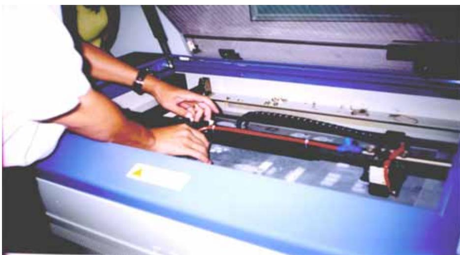
**Step3 :** Cut 25mm (1 inch) off the air assist tube on the original lens carriage.
